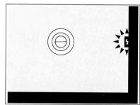
finder. When the SCA396 module is connected, the camera's focal plane shutter will automatically set at 1/60 sec, and ignore the settings on the shutter speed dial between 1/60 to 1/1000, including A and AEL. Slower shutter speed settings, however, (1/30 to 4 sec.) are not affected and will allow flash synchronization.
