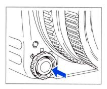
To use the Self-Timer, set the Shutter Release Selector to ⊗ and press the Shutter Release Button.
