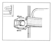
With your fingers, pull the Neck Strap Fastener (A) of the attaching clip upward and push part (B) in the direction of the arrow. The strap can now be removed
