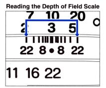
In addition to visual observation, the Depth of Field can be determined by using the Depth of Field Scale on each lens. f/stop numbers appear on both the right and left side of the red index mark in the center of the scale ring. Simply read the figures which appear above the f/stop numbers on the distance scale of the lens.
