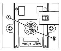
The Mamiya 645 PRO TL Tripod Socket accepts a standard 1/4" tripod mounting screw. For use with tripods having 3/8" mounting screws, first unscrew the small black philips head retaining screw in the center of the tripod socket. Then remove the 1/4" bushing with a thin coin. To re-install the 1/4" bushing, reverse the process.
