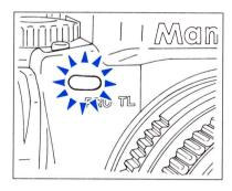
The Battery Check Lamp will light for 8 seconds and blink for 2 seconds, whereupon the shutter will go off.
