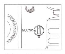
Aligning the white dot of the Multiple Exposure Lever with the vellow "MULTI" square, disengages the multiple exposure prevention mechanism, and the film will not advance after an exposure is made and the Film Advance Crank is turned
