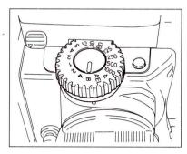
\* "B" can be terminated by shifting the Shutter Release Selector from (5) or the Shutter Speed Dial from "B".
