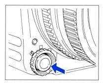
For time exposures set the Shutter Release Selector to 🖒, the self-timer mode, and set the Shutter Speed Dial to "B". Press the shutter release and both mirror and shutter will stay open until the shutter release is pressed again. You may also use a cable release together with the cable release adapter. (The battery circuit will automatically switch off to save power.)
