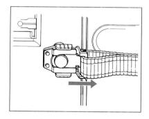
2. Place the hole of the strap fastener (A) over the Neck Strap on the camera body as illustrated, and pull until it clicks and locks into place.
