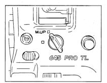
This is an important feature when the tripod mounted camera is used at slow or long exposure times and particularly also with use of long telephoto lenses. It eliminates the possibility of even the slightest "mirror bounce" which may affect image sharpness.
