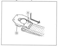
**1.** While pushing down, pull out the Neck Strap Fastener (A) of the attaching clip.
